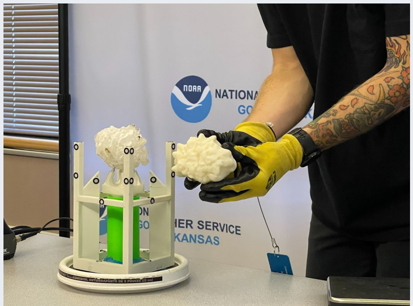
An IBHS expert measures the Kirk hailstone using a 3D laser scanner while visually comparing it to the Bethune hailstone in his hand.
